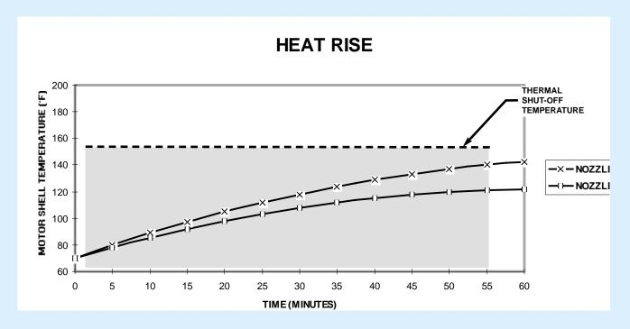
The motor driving this pump has a built in thermal protector that will open, shutting off the pump, when the surface temperature of the motor heats to approximately 150°F. Motors of this size and construction require 15 to 30 minutes of cooling time before the thermal protector closes and re-energizes the pump. Lower current levels heat more slowly, allowing longer run times, but the cool down time still averages about 30 minutes, at 70°F ambient temperature.
