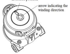
cable rewinder handle in working position
