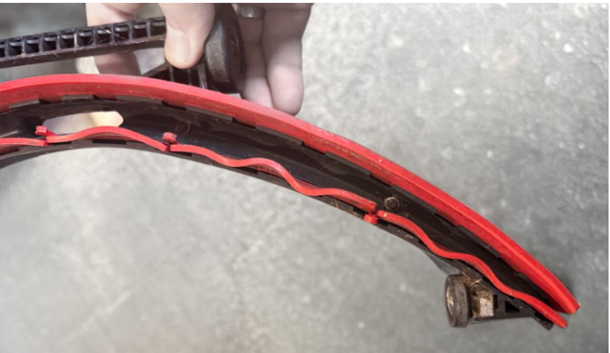
Wavy Squeegee caused by grease or oil
