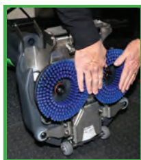
1. PLACE THE TWO BRUSHES ONTO BRUSH DRIVE (SIMPLY PUSH ON)
