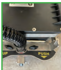
8. PRESS DOWN 'PUSH' TO LOWER SQUEEGEE ASSEMBLY
