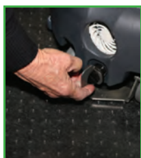
1. EMPTY THE SOLUTION TANK. BY USING SPANNER SUPPLIED. TURN ANTI CLOCKWISE TO UNSCREW, REMOVING PLUG AND FILTER
