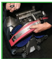
2. FIT SQUEEGEE ASSEMBLY WITH TWO WINGNUTS SUPPLIED
