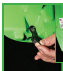
6. REMOVE DRAIN PLUG TO SAFELY RELEASE WASTE & RINSE TANK (WIPE AWAY ANY EXCESS GRIME)
